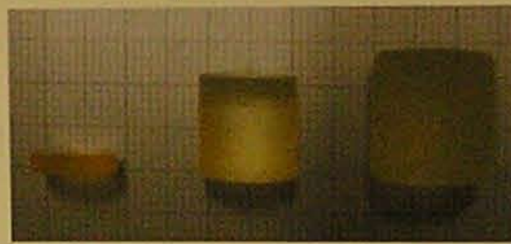
Figure 5. Expansion of a compressed hydrogel (compression ratio 3), before, during, and after expansion.
