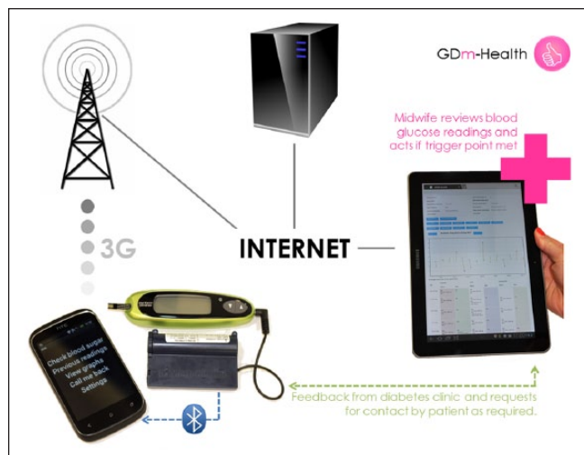
Figure 1. Diagram of m-health system for the management of gestational diabetes mellitus (GDM).
